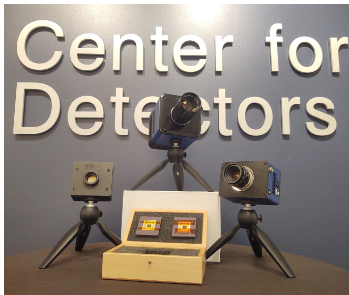
Figure 1. The image shows four different QIS systems: the QIS pathfinder (left), QIS.CDK REV2 (top) and REV1 (right), and two of three chip carriers with QIS for cryogenic testing (bottom).
