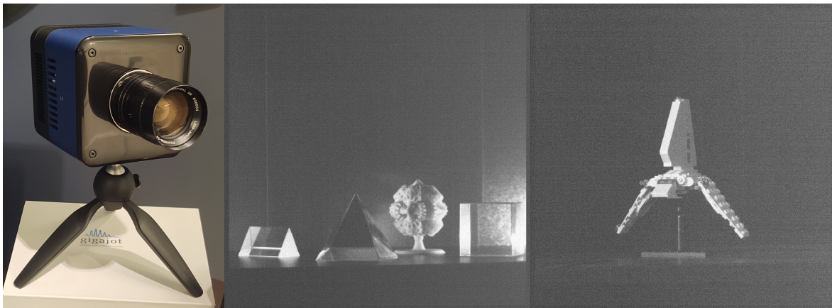
Figure 4. The QISCDK REV2 camera with an attached off-the-shelf lens (left) and two images of objects under low-light conditions (right). The mean signal in the image is 0.16\text{ e}^-/\text{pix} with bright regions reaching up to 3.3\text{ e}^-/\text{pix} .
