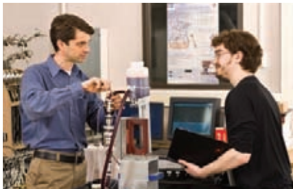
Pumping Blood: Dr. Steven Day and Steven Snyder, 2nd year mechanical engineering student, test the left ventricular assist device (LVAD) to assess the damage to red blood cells caused by flow within the pump.
