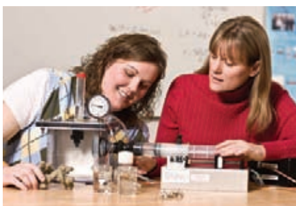
Realistic Model of Alveolar Sac: Emily Berg, 6 th year mechanical engineering graduate student, and Dr. Risa Robinson use an anatomically accurate 3-dimensional model of an alveolar sac to complete the first-ever study that compares fluid flow in healthy and diseased lungs. The study aids in the understanding of the physiological conditions that affect particle deposition and absorption into the blood stream.
