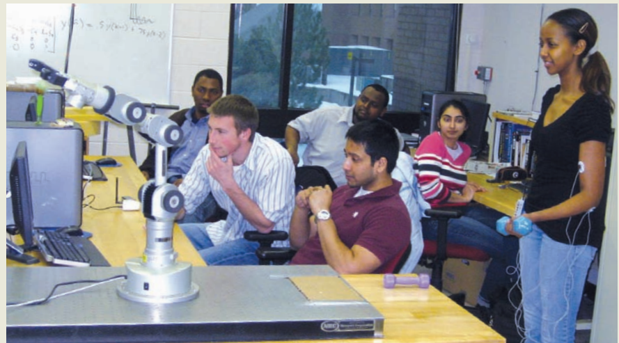
Testing Bio-Electronic Device: Adey Gebregioris, 5 th year electrical engineering student, controls a robotic manipulator using sEMG signals obtained from her bicep muscles. Here, Gebregioris is curling her arm and the robot is imitating the action.
