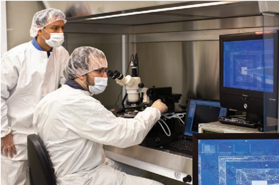
Probing a Test Structure: Matthew Simpson (right), 4 th year biotechnology student, and Dr. Donald Figer (left) work in the clean room probing a test structure to determine properties of the detector, like dark current levels and breakdown voltage.
