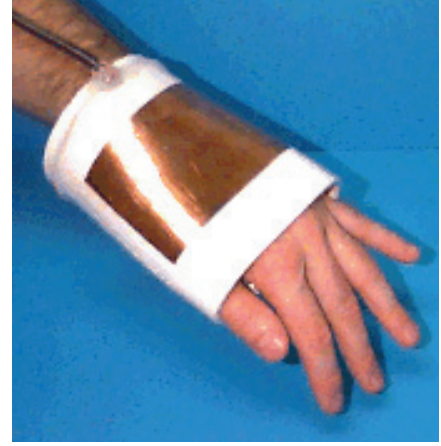
MRI Coil for the Extremities: RIT Professor Joseph Hornak was part of a team that developed an asymmetric single-turn solenoid style MRI coil, as shown on the right. The device is especially suitable for MRI of the human wrist.
