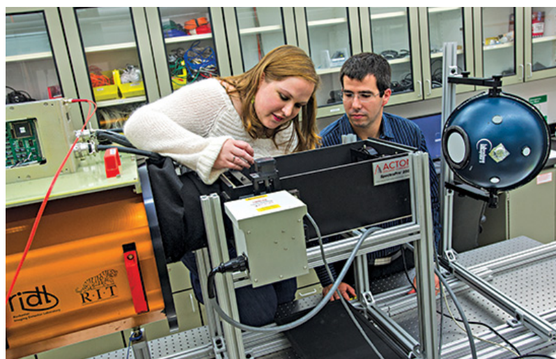
Kim Kolb, a Ph.D student in the Chester F. Carlson Center for Imaging Science, and Brandon Hanold, an engineer in the Center for Detectors, prepare to test one of the detectors grown on silicon wafer substrates.
