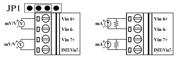
**Note**: When connecting to a current source, an optional external 125-ohm resistor is required.
