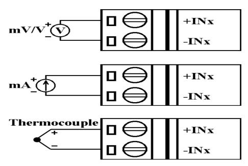
**Note**: When a channel is connected to a current source, the corresponding jumper should be shorted, see Section 1.7.2 for details.
