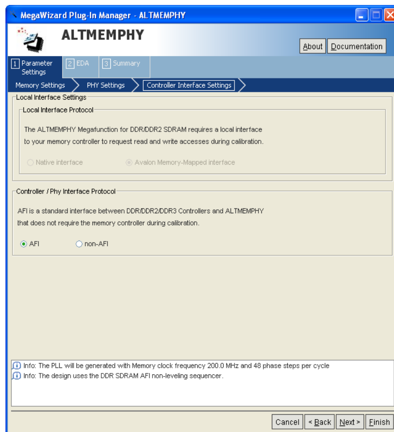
Figure 2-8. Controller Interface Settings
