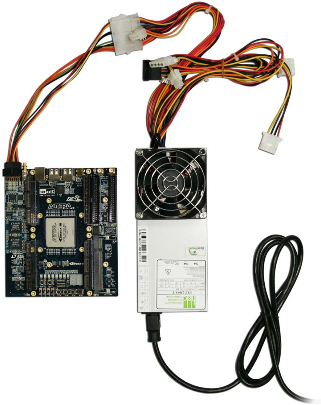
Figure 7. The connection setup for DE3 board and power supply
