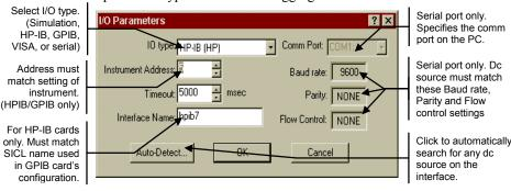
If there seems to be no communication between the Agilent 14565A application and the dc source, select **Auto Detect** to detect any dc sources connected to your computer. If you still cannot communicate with the dc source and you wish to exit the application, select **Simulation** mode in the IO type field. Then exit the application.
