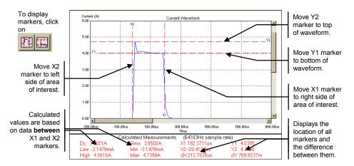
You can also zoom in on a specific area of the waveform. Zooming in only rescales the display, no calculations are performed in the zoom area.
