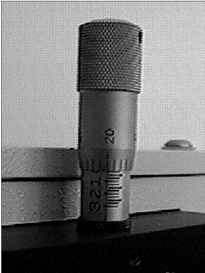
Slit Width Setting: 200 Micrometers (0.200mm)
